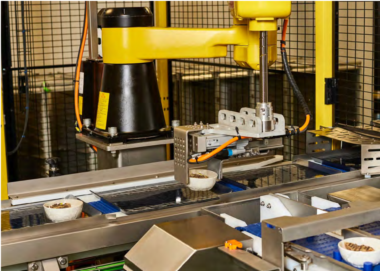
A robot at Delta's kitchen assembles food trays with cutlery, napkins and side dishes. Photographer: Bailey Garrot for Bloomberg Businessweek
